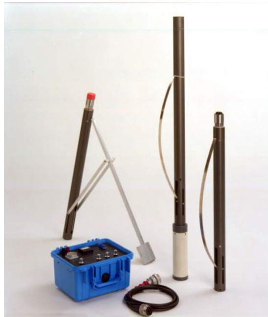
Figure 11: Geostuff BHG borehole receiver system
