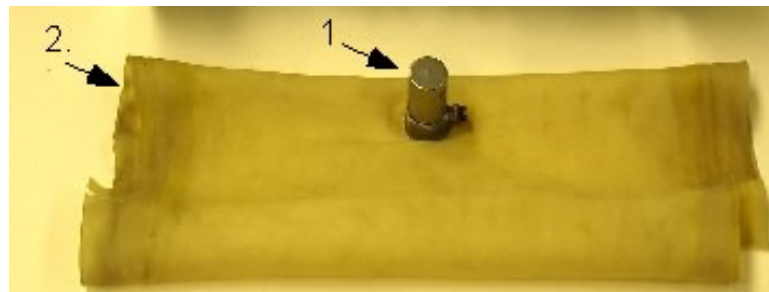
Figure 39: Accelerometer (1) on initial latex membrane (2). (Kalinski, 2012)
